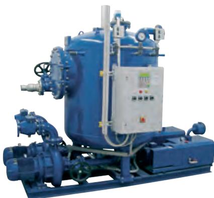
In the Roediger® vacuum station, the wastewater is collected in a wastewater tank and then conveyed with wastewater discharge pumps into a conventional gravity sewer main or directly into a wastewater treatment plant. Vacuum pumps in the vacuum station generate the negative pressure required in the pipe network.
