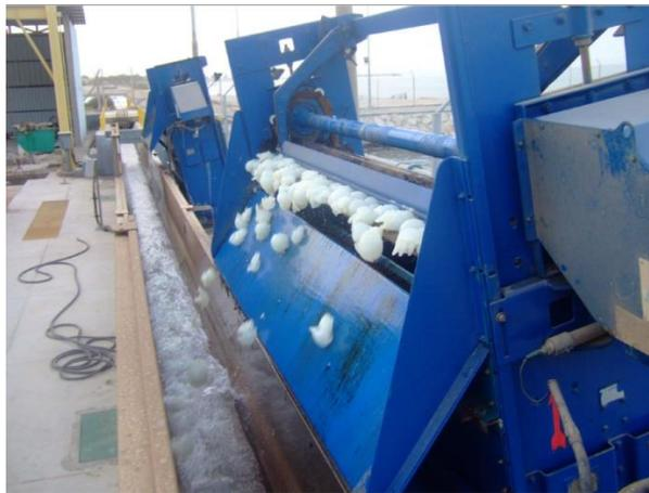
**Figure 3.** Power and MSF-Desalination Plant - Qurrayah, Kingdom of Saudi Arabia. Upgrading with 20 Revolving Chain Screens (by Aqseptence Group), thus removing up to 60 t/h jellyfish per machine out of sea at a total flowrate of 700,000 m<sup>3</sup>/h; material of construction of submerged parts is 316L with impressed current cathodic protection
